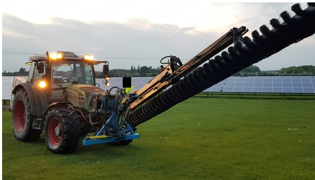
Plate 2-15: Tractor-Mounted Cleaning System
